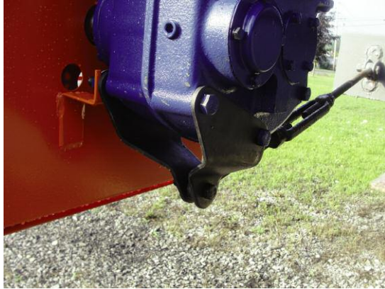
Torque Arm Included With Shaft Mount Reducer
